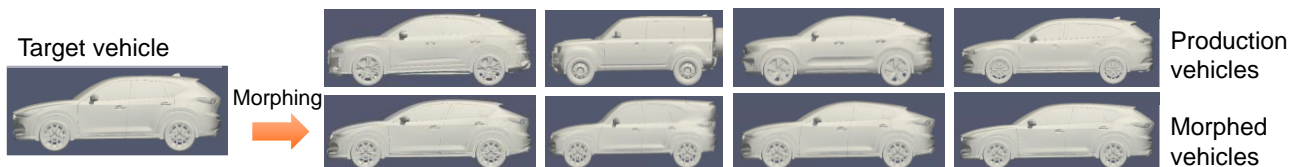
Fig. 2.2.1-8 Comparison of sideview of production cars (top) and the target vehicle morphed to have similar proportions and silhouette (bottom)
