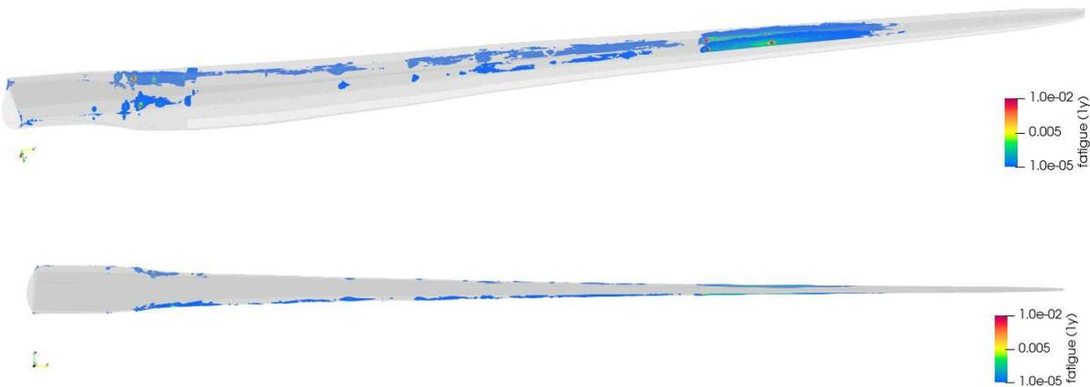
Fig. 2.5-2. Distribution of annual accumulated fatigue damage for turbulent inflow of TSR=6.
