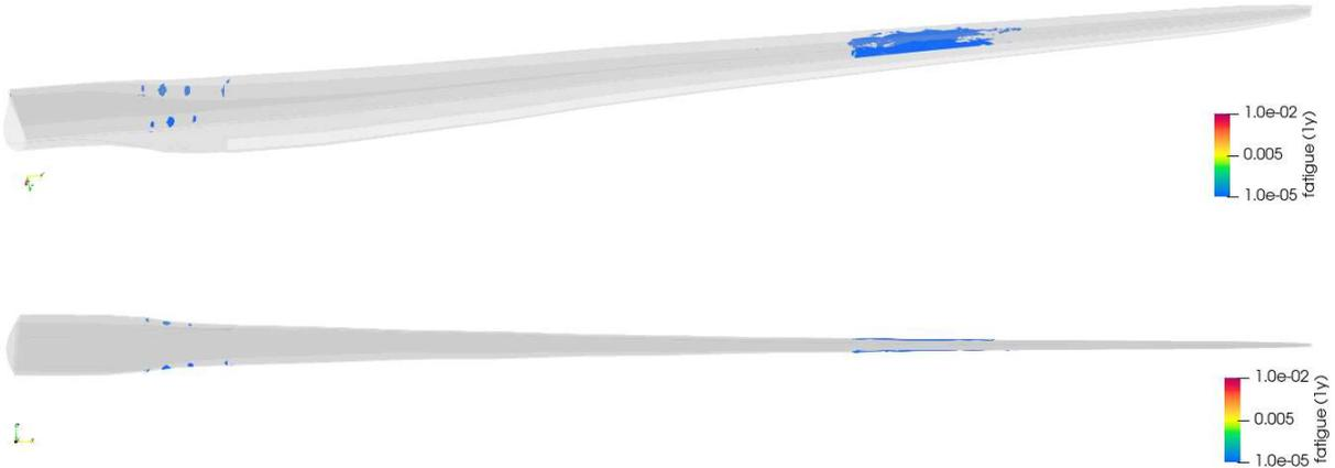
Fig. 2.5-3. Distribution of annual accumulated fatigue damage for turbulent inflow of TSR=7.
