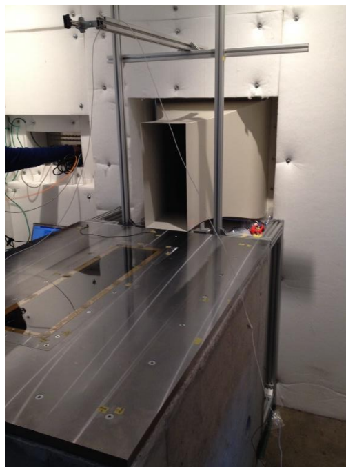
Fig. 2.2.5-28 Picture of experimental set up of wind tunnel for vehicle interior noise.
