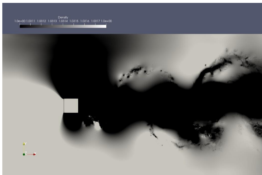
Fig. 2.2.5-12 Density field around a square cylinder.
