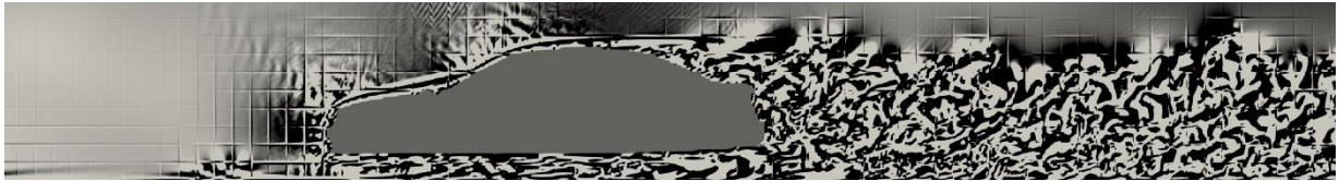
Fig. 2.2.5-18 Sound field around an automobile simulated by FFX, Re=Re_0/300 .
