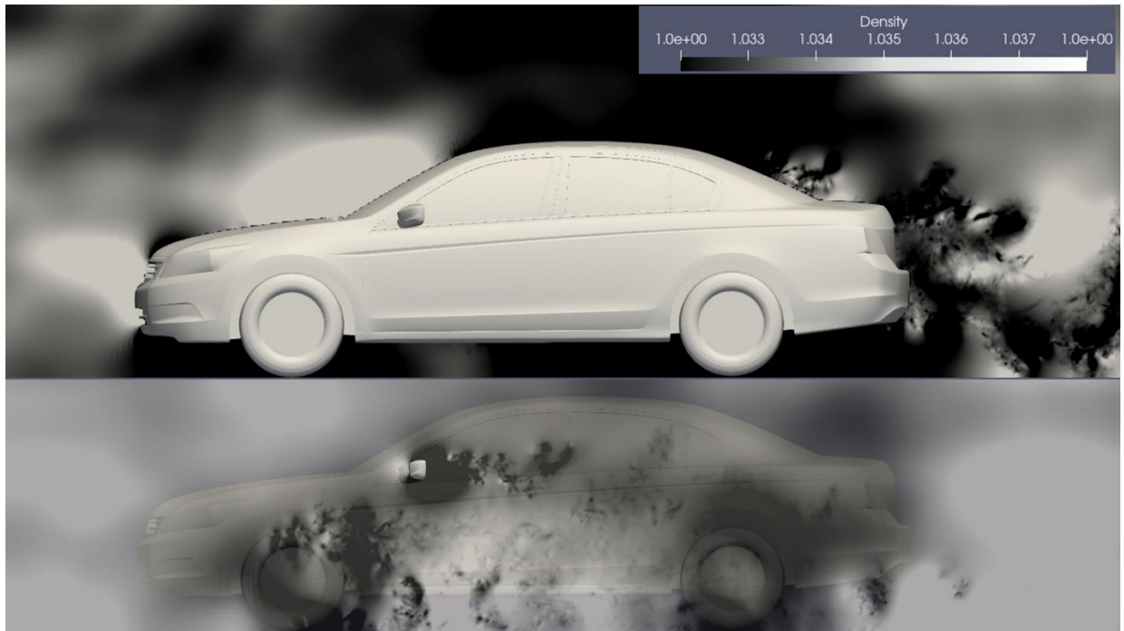
Fig. 2.2.5-24 Sound fields around an automobile simulated by FFX, Re=Re_0/40 .
