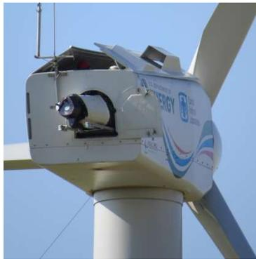
(b) DTU spinner LiDAR
