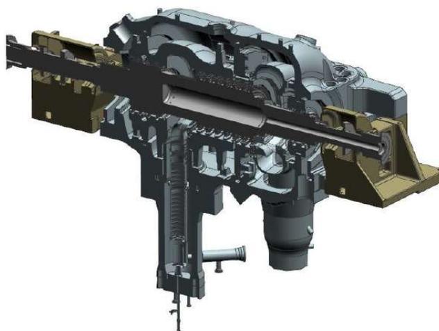
Figure 4.2.1-1. Supercritical CO<sub>2</sub> turbine and combustor [1]
