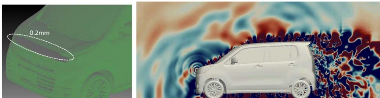
Fig. 4.2.2-5 The computational grid overview (left) and the propagation of the pressure fluctuation (right).
